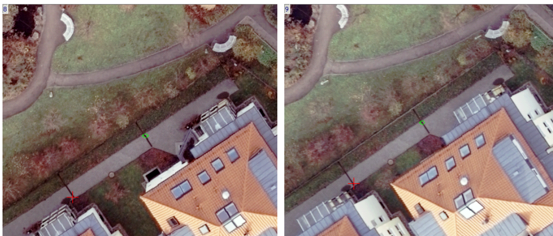
Fig. 94. The left image shows triplet point, located in the center of triple overlap area, the right one – triplet point from the right image
